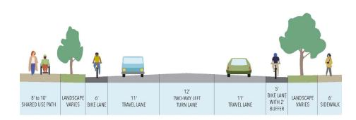
Example design of road width and right-of-way
